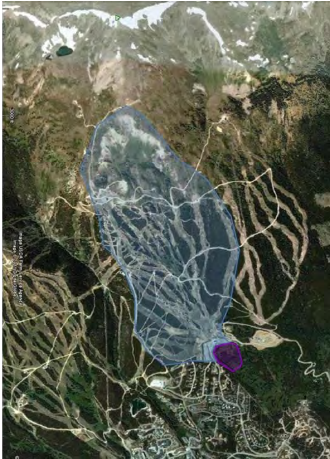
Figure 60: The contributing watershed (blue) to the Cucumber Gulch Preserve (purple) is entirely within the Breckenridge Ski Area and severely modified to meet that purpose
